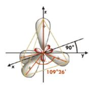
The angle of 109°28' - tetrahedron angle (= the double of the angle between the cubic diagonal and the edge of the cube) - between the connecting lines of two neighbour atoms derives as well geometrically from the crystal structure as from the orbits of the four electrons of the carbon atom's second layer that are sp3 – hybridised (a paired selectron mutates to an unpaired p-electron).
